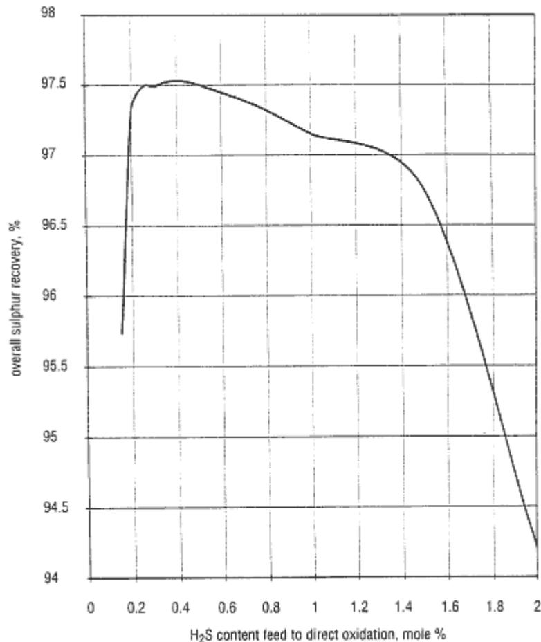
Figure 3. Overall sulphur recovery vs H<sub>2</sub>S content in feed to direct oxidation.
