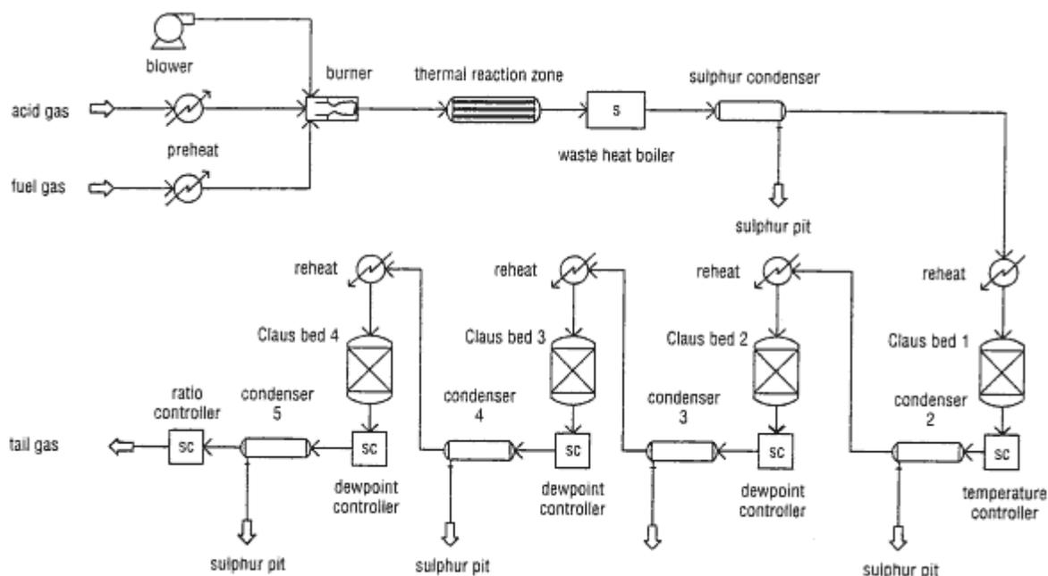
Figure 1. Process flowsheet for Example 1.
