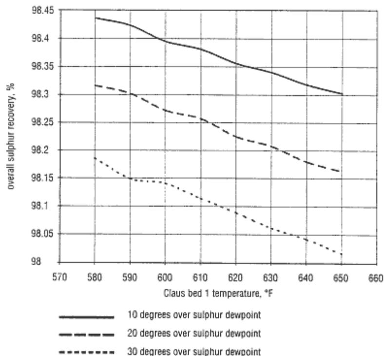
Figure 2. Overall sulphur recovery vs bed 1 temperature at constant bed 2 and 3 temperatures.
