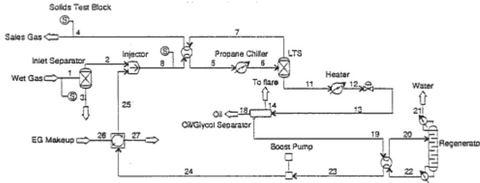
Figure 2. Typical glycol injection unit.
