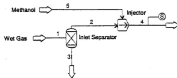
Figure 3. Typical methanol injection unit.
