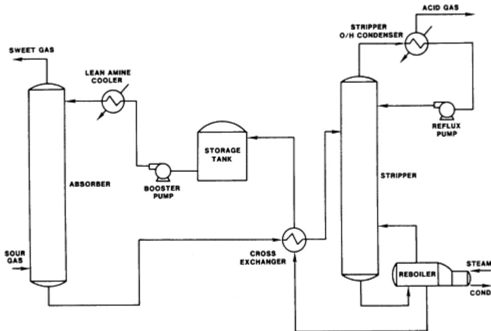
Figure 1. Process flow sheet for common sweetening plant.
