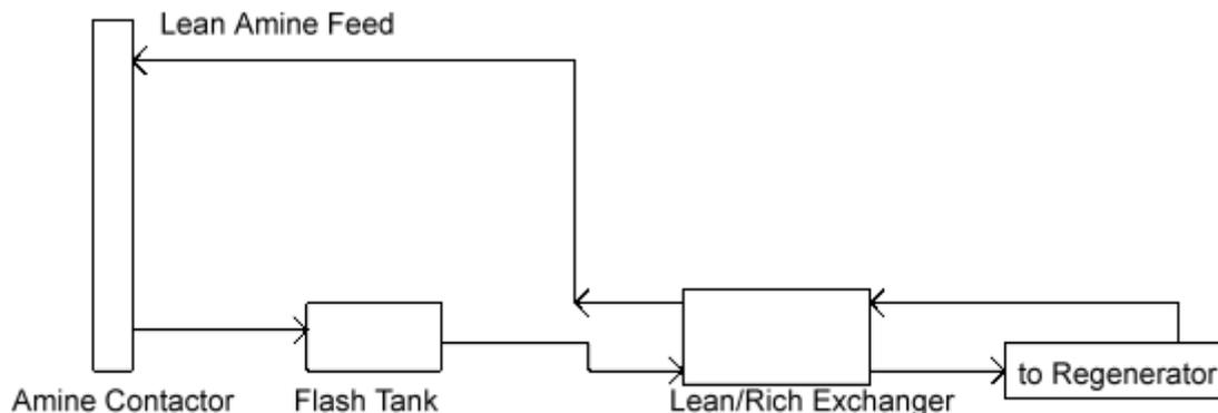
Figure 1. Current amine treating loop without BTEX-T.rex process.
