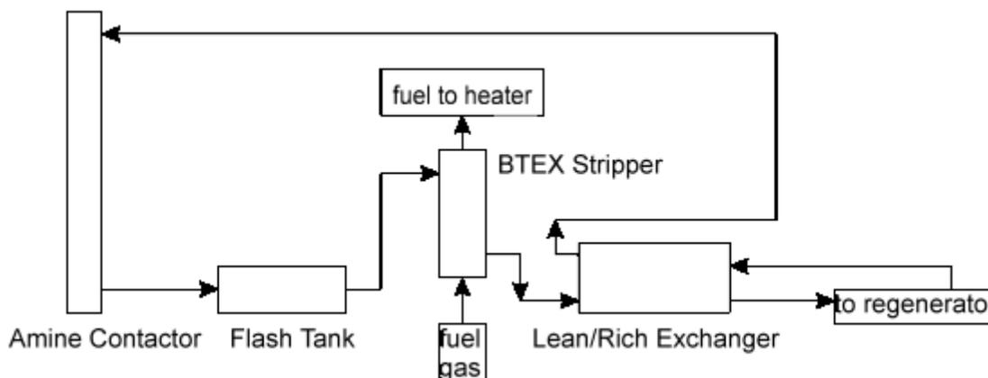
Figure 2. Amine treating loop with BTEX-T.rex process.
