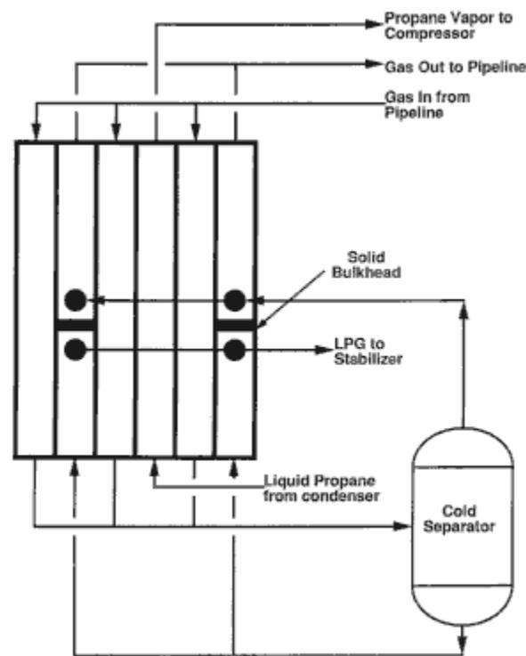
Figure 4. Detail process flow schematic for complex plate exchanger in Case 1.
