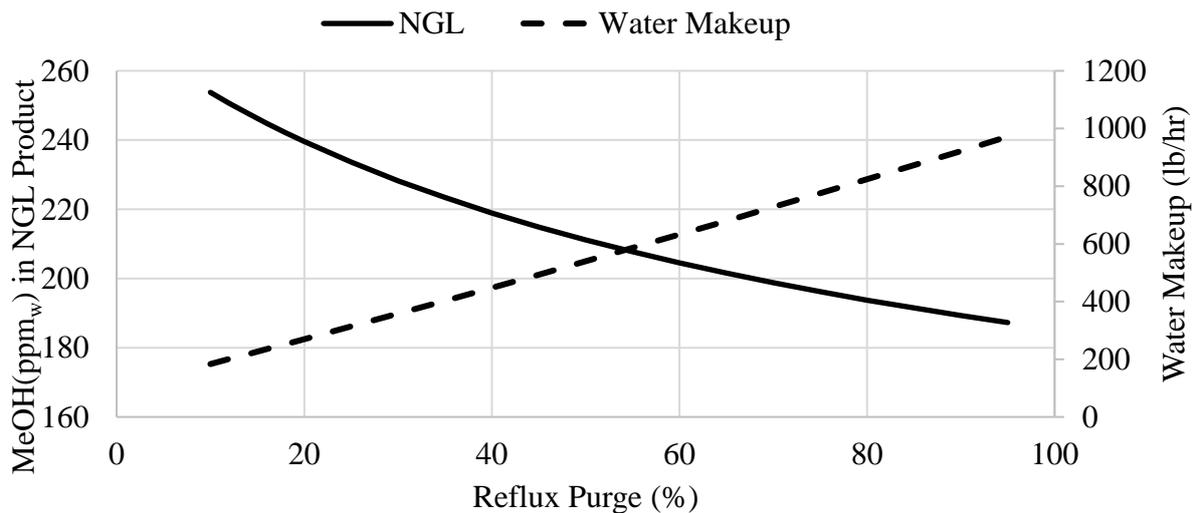
**Figure 7:** Reflux Purge Effect on Methanol in the NGL and Water Makeup
