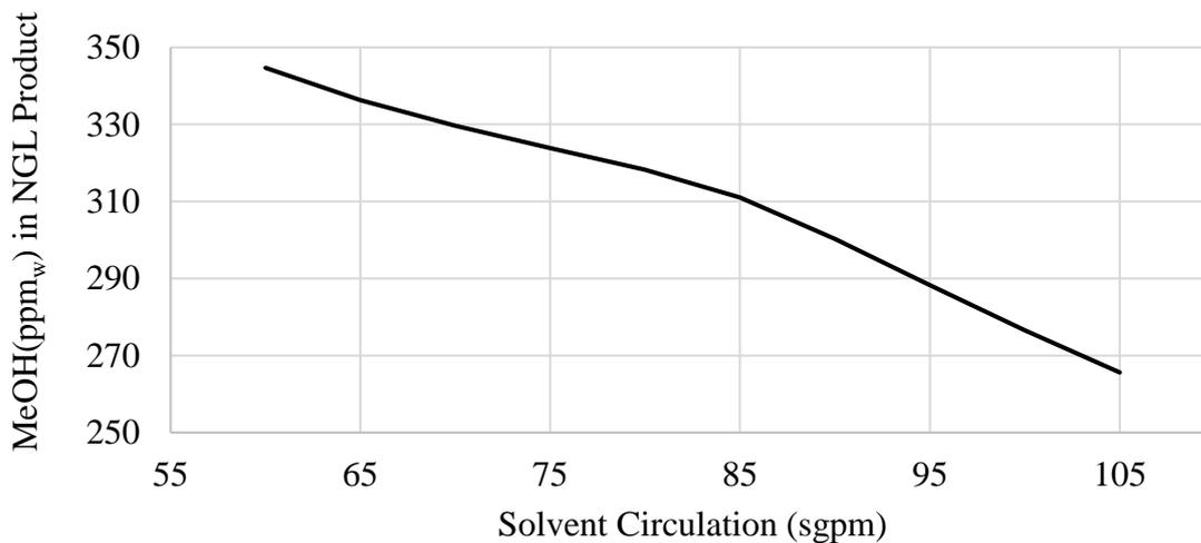
**Figure 4:** The Effect of Solvent Circulation Rate on NGL Methanol Content
