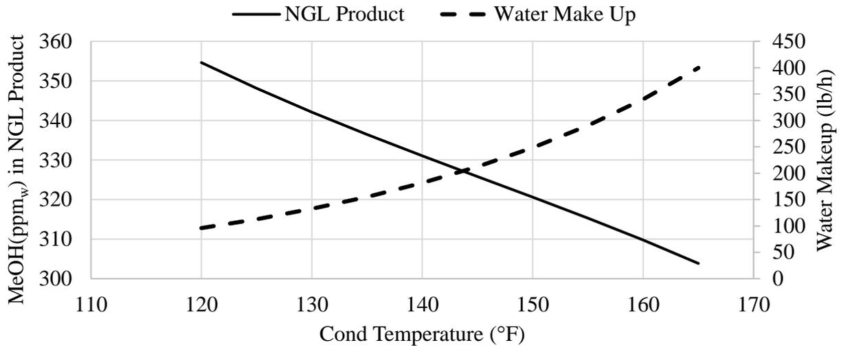
**Figure 3:** NGL Methanol Content and Water Makeup vs. Condenser Temperature
