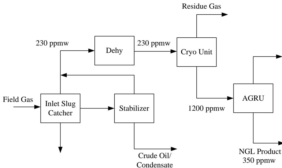
*Figure 1: Methanol Concentrations in the Texas Gas Processing Plant*
