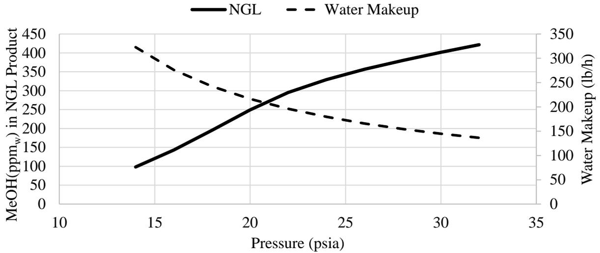
**Figure 6:** Stripper Pressure Impact on Methanol in the NGL and Water Makeup
