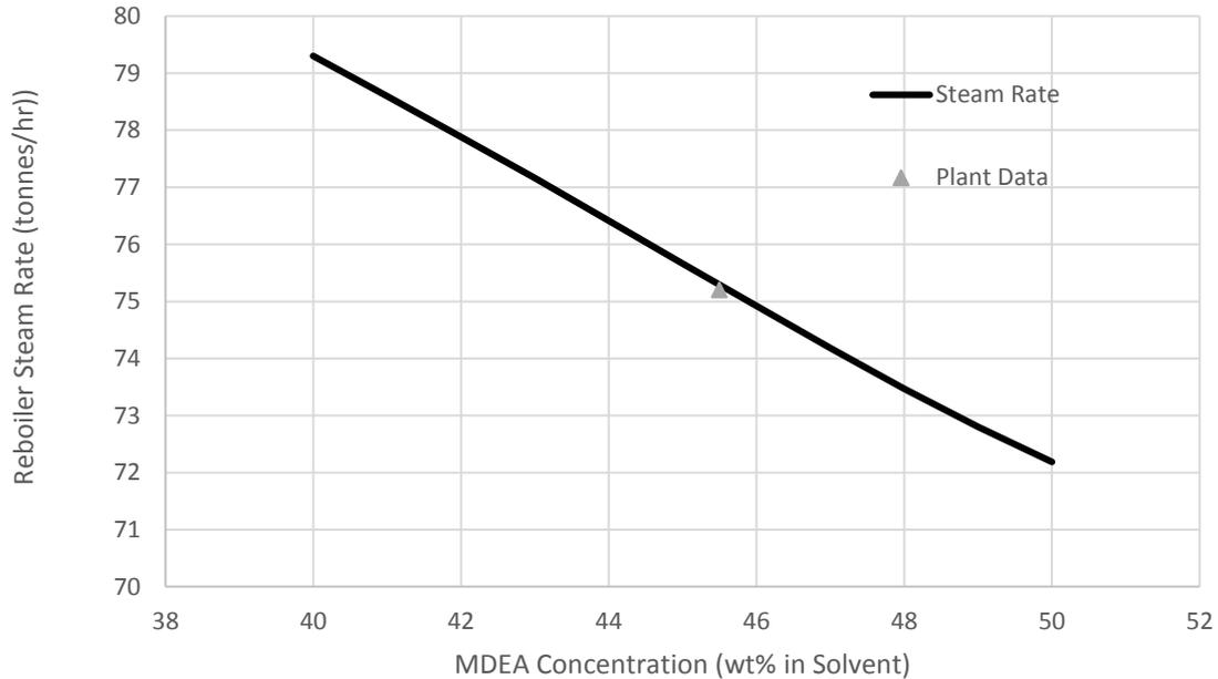
**Figure 4:** The Effect MDEA Concentration has on the Reboiler Steam Consumption Rate
