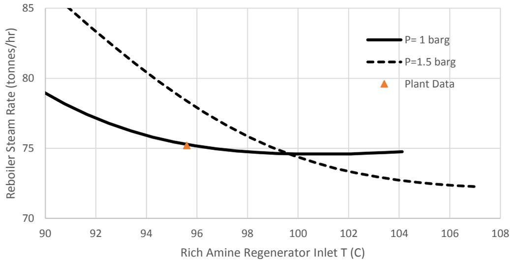
**Figure 5:** The Effect the Lean/Rich Exchanger and Regenerator Pressure Have on the Reboiler Steam Consumption
