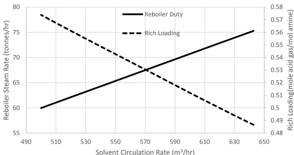
**Figure 3:** The Impact of Solvent Circulation Rate on the Reboiler Steam Consumption and Rich Loading
