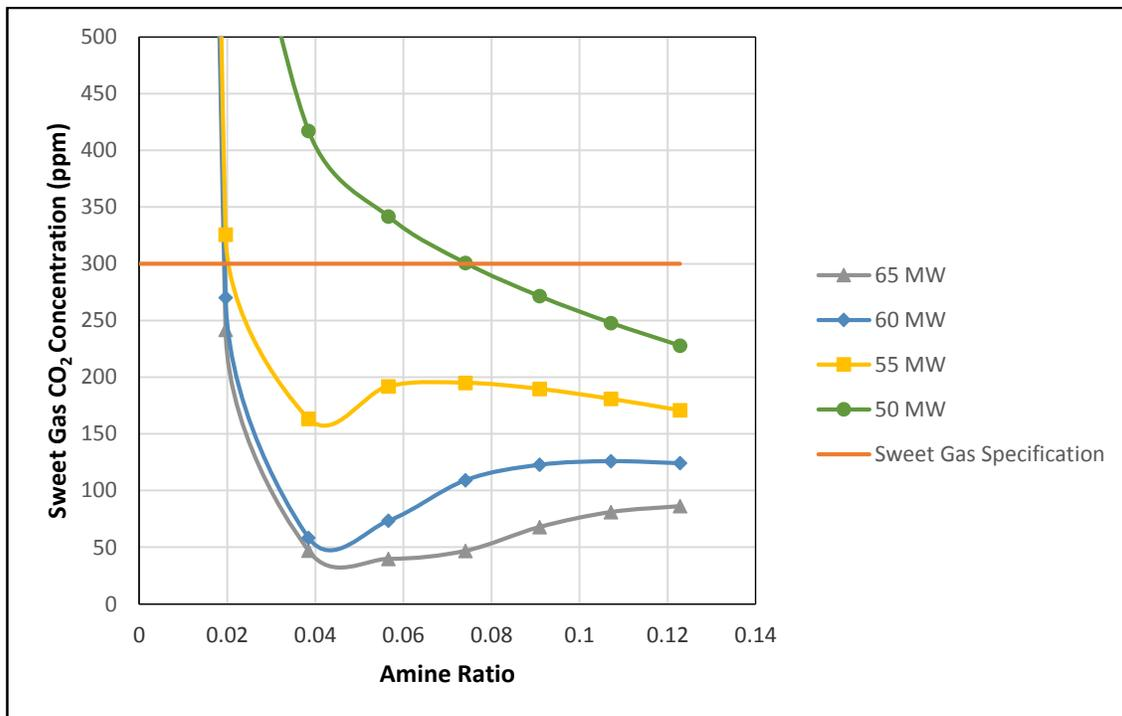
**Figure 3: Absorber Performance for Various Amine Ratios**
