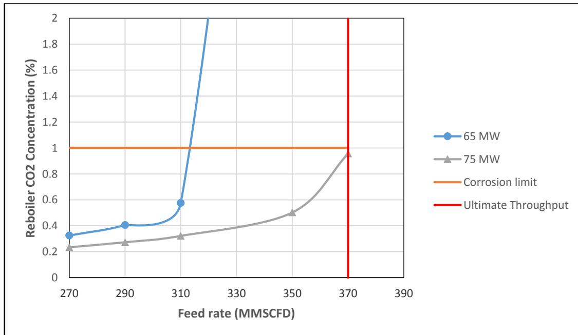
**Figure 9: Effect of Reboiler Duty on Reboiler Vapor CO<sub>2</sub> Concentration**
