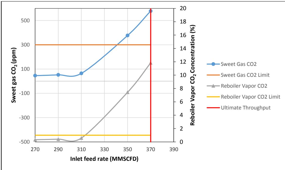
**Figure 7: GSP#5 Amine Absorber Performance at 65 MW and 0.53 Rich Loading**
