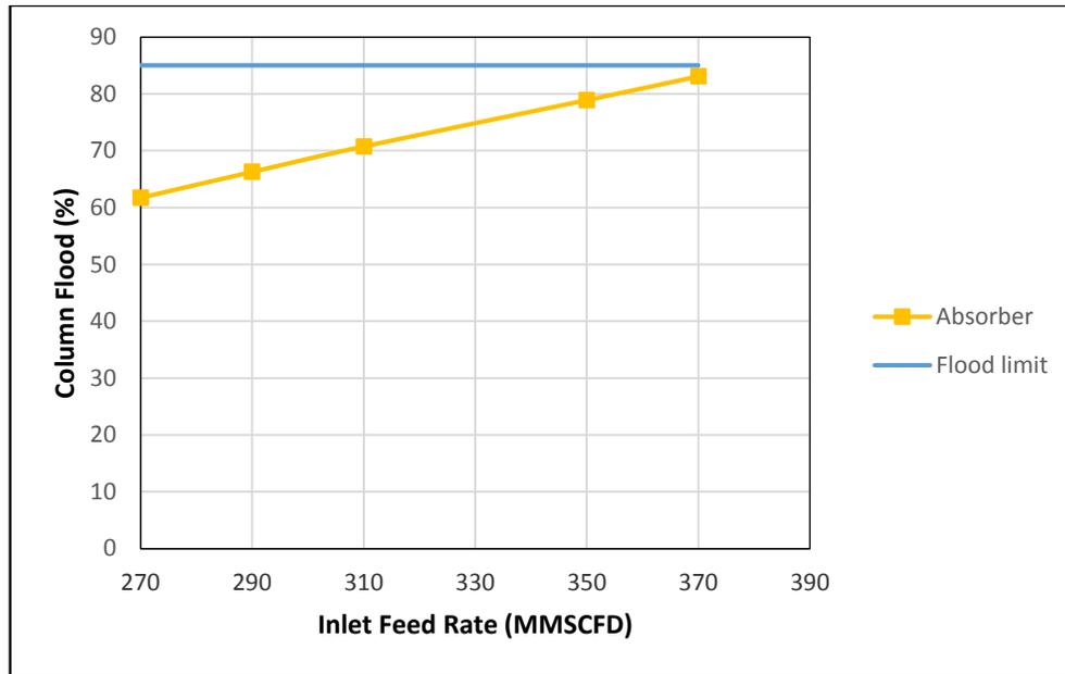
**Figure 5: Amine Absorber Capacity**
