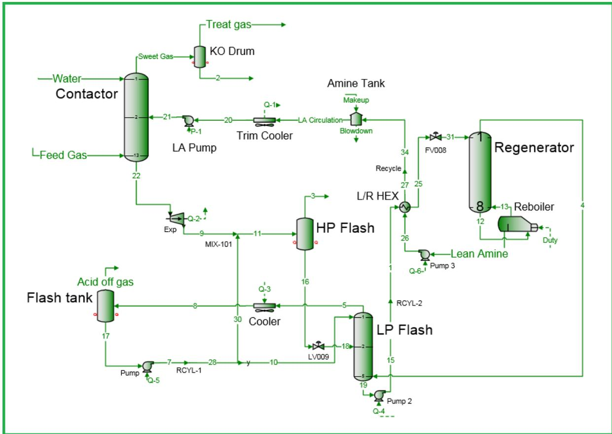
Figure 1: Process Flow Diagram for PTT GSP#5 Amine Sweetening Unit.
