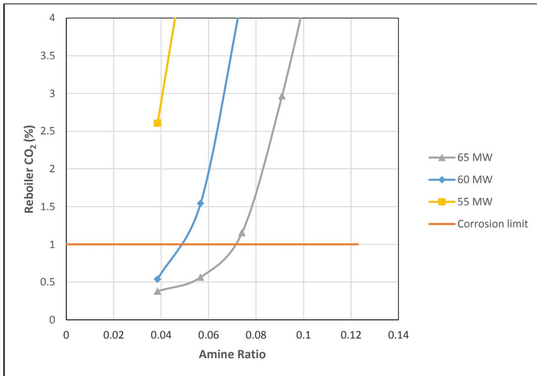
**Figure 4: Reboiler Vapor CO<sub>2</sub> Concentration versus Amine Ratio**
