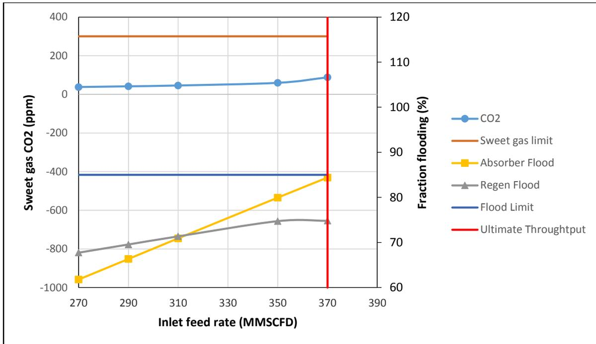
**Figure 8: GSP#5 Amine Absorber Performance at 75 MW**
