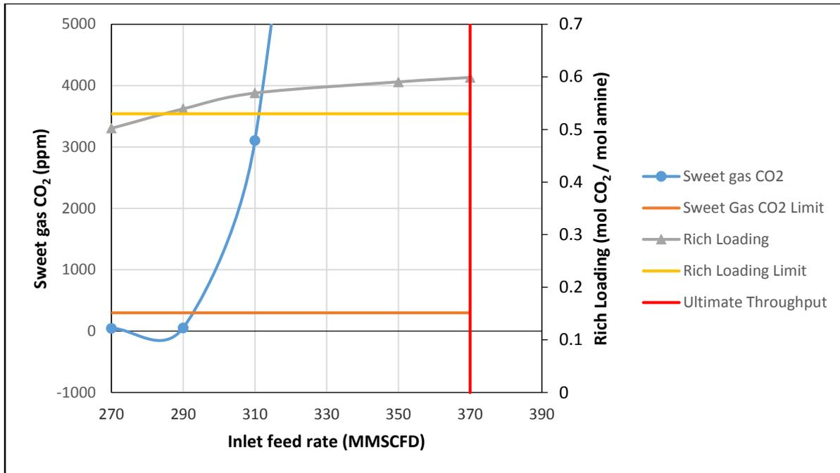
**Figure 6: GSP#5 Absorber Performance at Maximum Pump Capacity**
