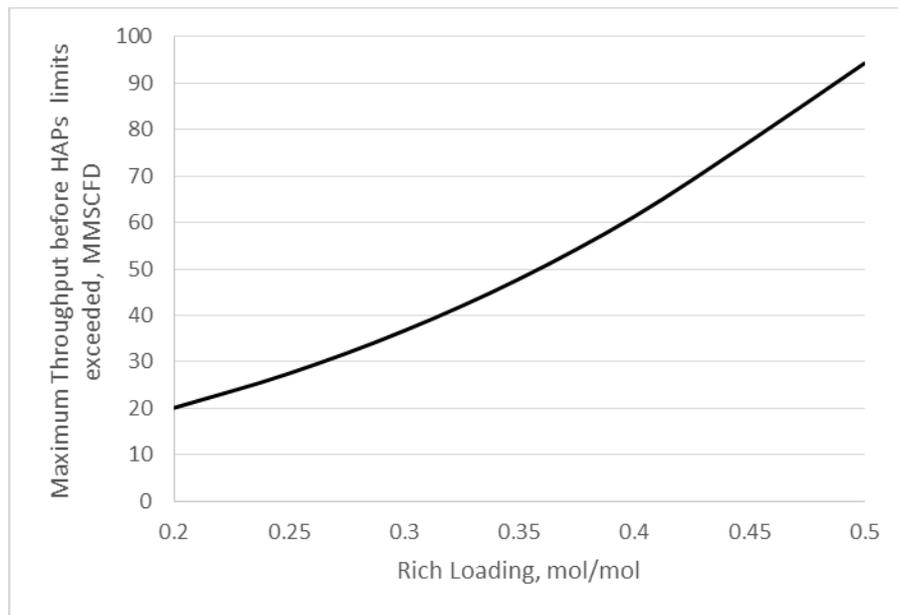
**Figure 1:** Effect of Over Circulation on BTEX Emissions from an MDEA unit, 0.25% BTEX in feed gas
