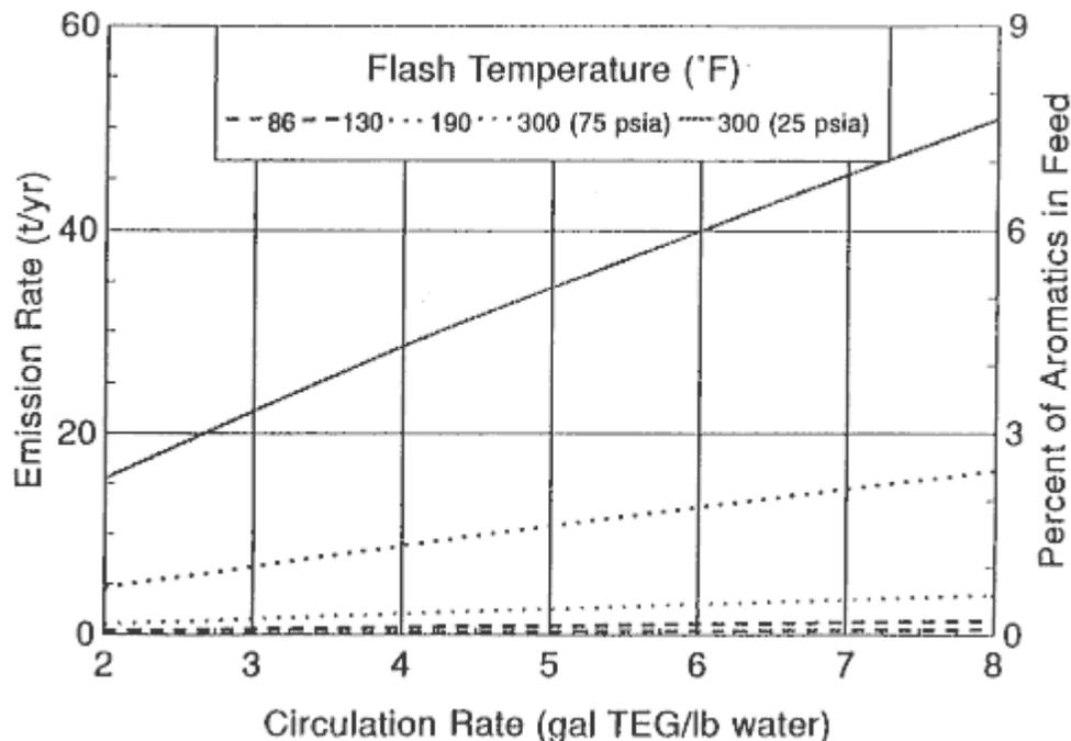
Figure 5. Aromatic emissions at the flash tank.
