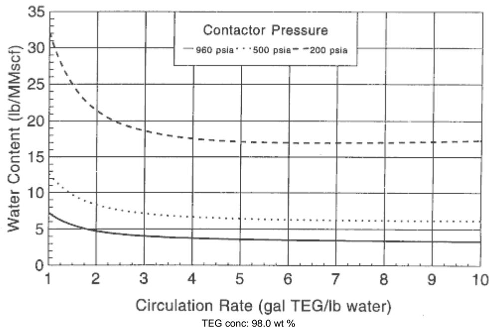
Figure 2. Residual water content of dry gas.
