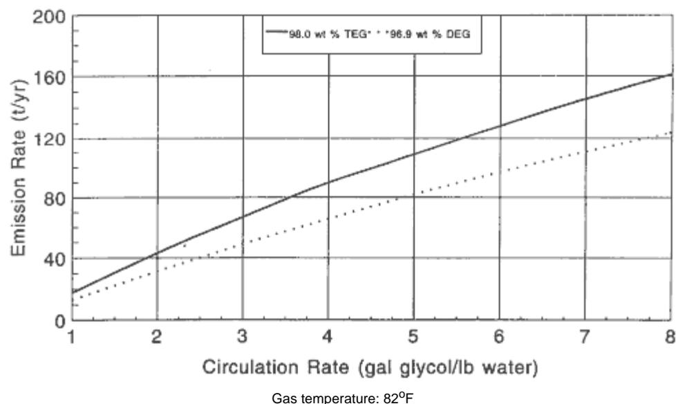
Figure 11. Total aromatic emissions for DEG and TEG units.
