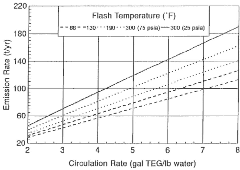
Figure 3. Non-aromatic VOC emissions from the flash tank.
