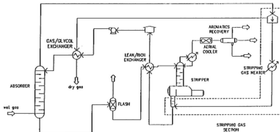
Figure 1. Typical glycol dehydration unit.
