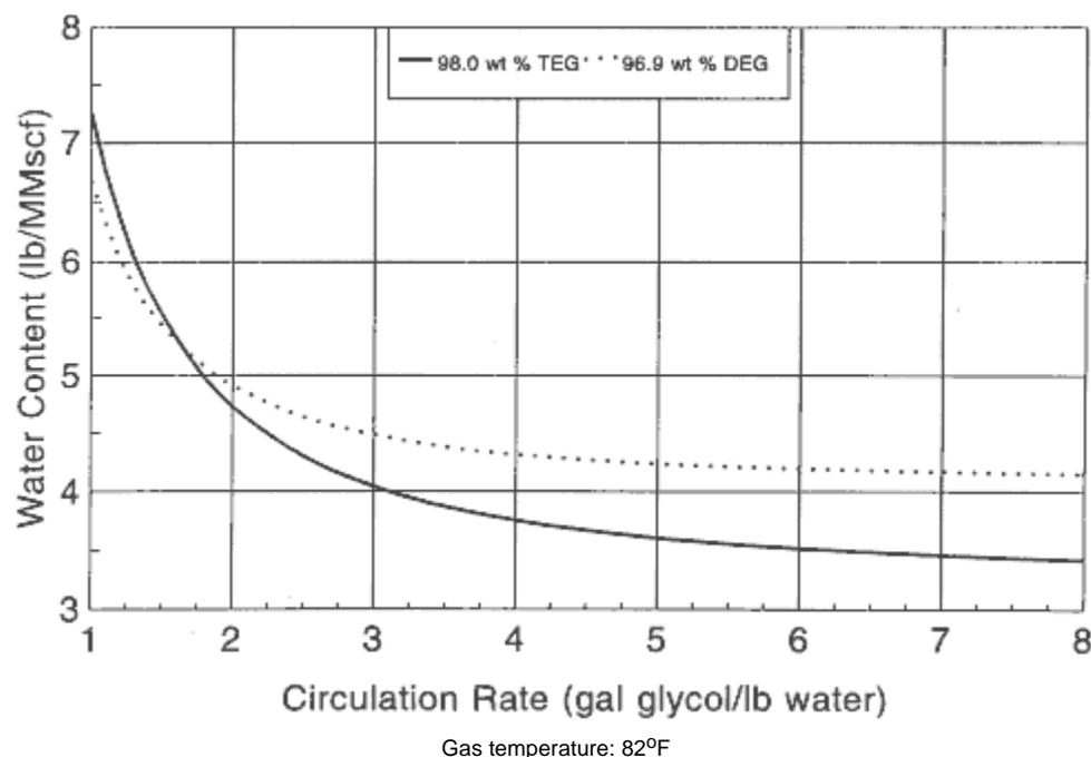
Figure 10. Residual water content of dry gas using DEG and TEG.
