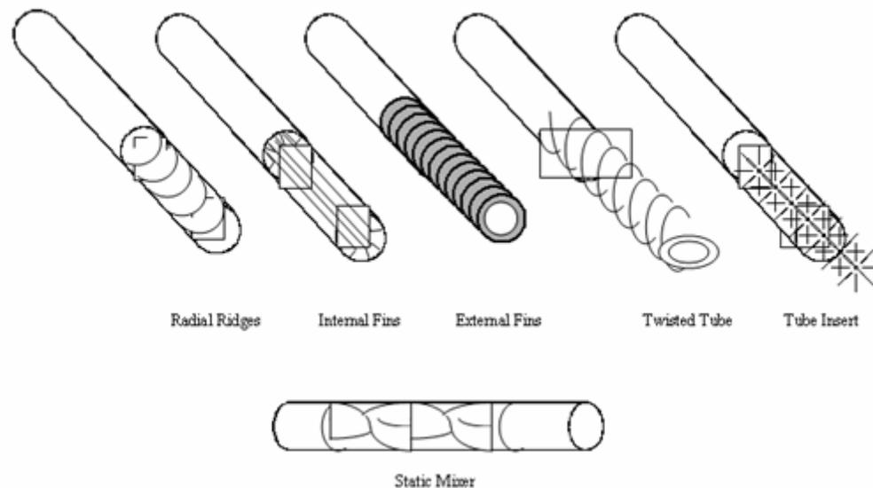
Figure 1. Examples of tubes with heat transfer enhancement.
