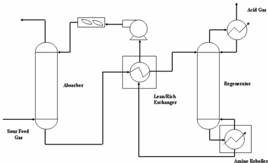
Figure 3. Schematic of a simple amine unit.
