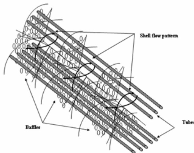
Figure 2. Schematic of helical baffles.
