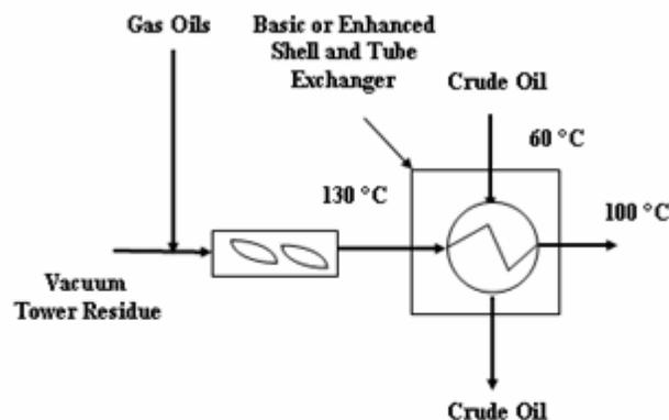
Figure 4. Schematic of a Crude Preheat unit.
