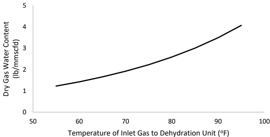
**Figure 8: Effect of Inlet Temperature on the Dry Gas Water Content for 390 °F Reboiler and 6 scfm Stripping Gas**
