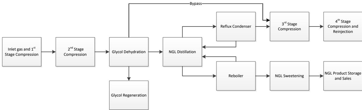
**Figure 3: Mabee Gas Plant Block Flow Diagram**
