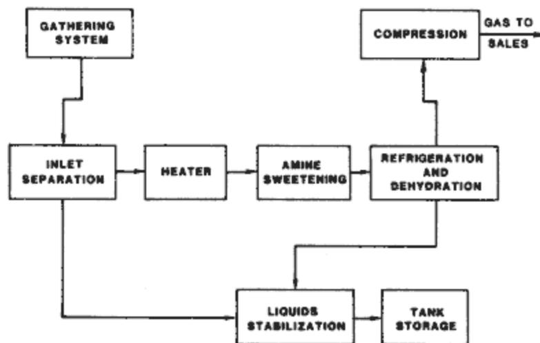
Figure 1. Block flow diagram for Forestburg Facility.
