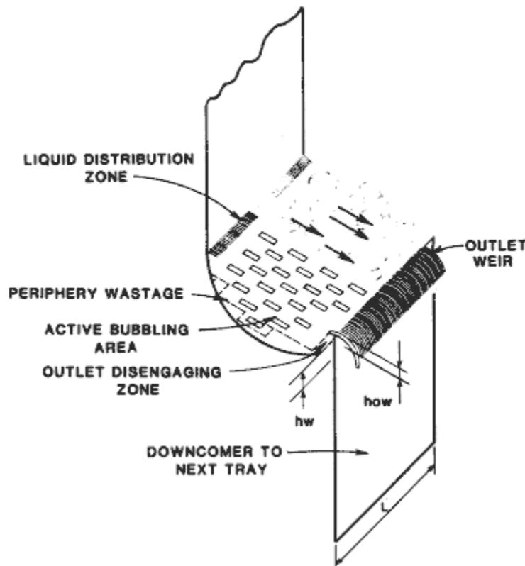
Figure 2. Typical contactor tray arrangement.
