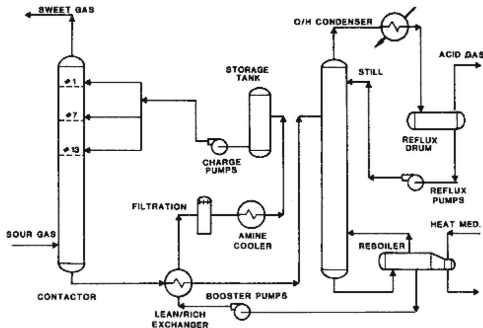
Figure 3. Process flow diagram for Forestburg sweetening plant.
