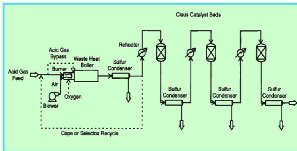
Figure 1. Schematic of the basic Claus process.
