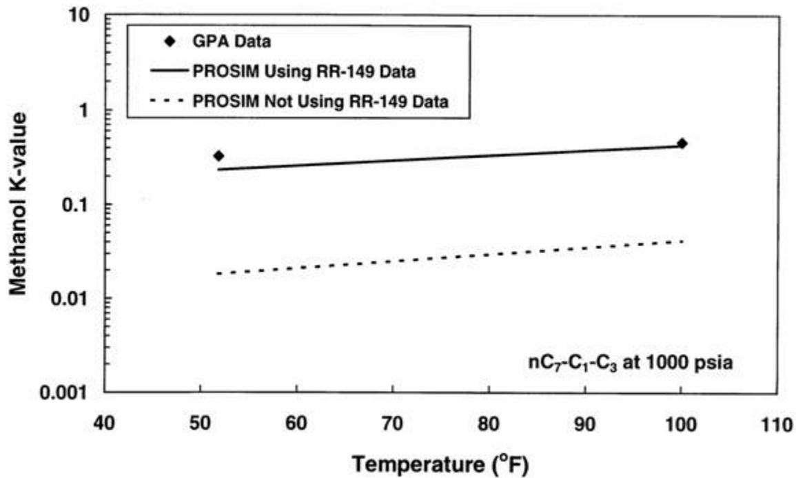
Figure 2. Methanol K-value improvement using RR-149 data for 25 wt% methanol
