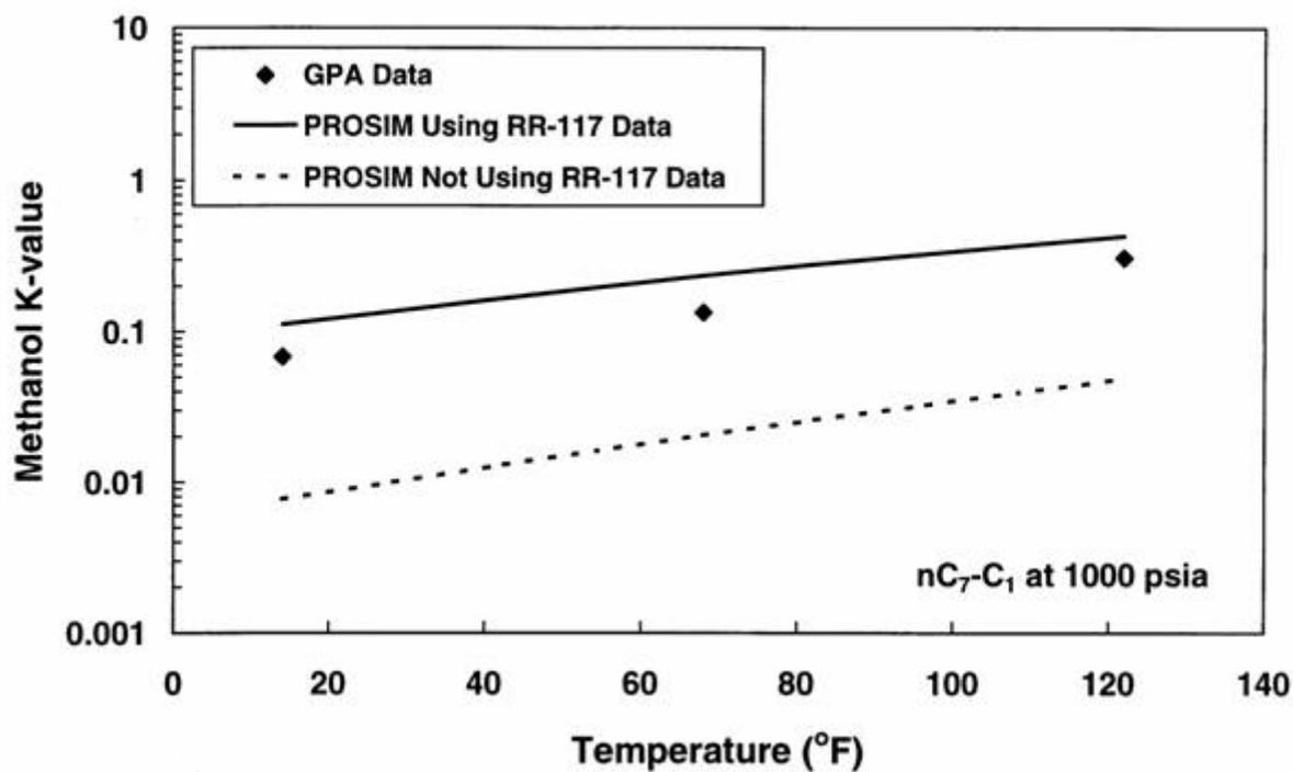
Figure 5. Methanol K-value improvement using RR-117 data for 70 wt% methanol.
