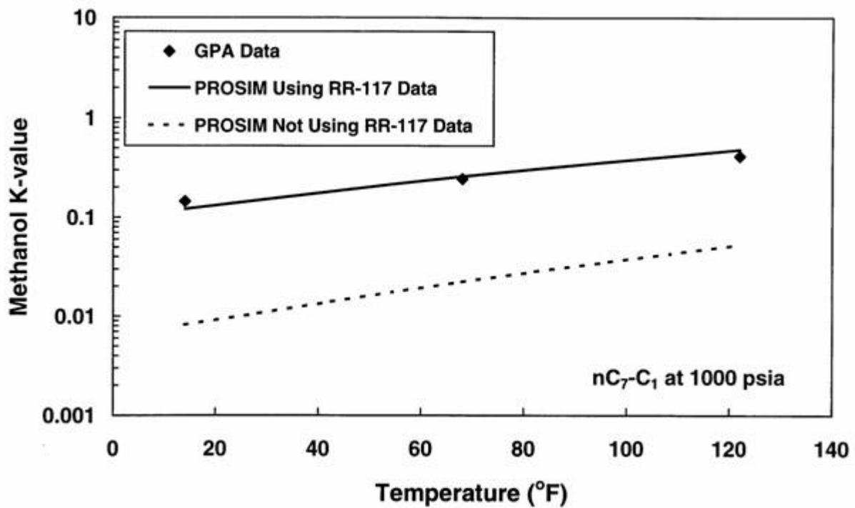
Figure 3. Methanol K-value improvement using RR-149 data for 50 wt% methanol
