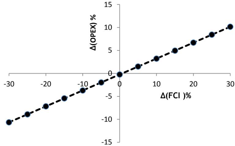
**Figure 5:** Effect of change in Fixed Cost Investment to Operating costs of ADGAS plant
