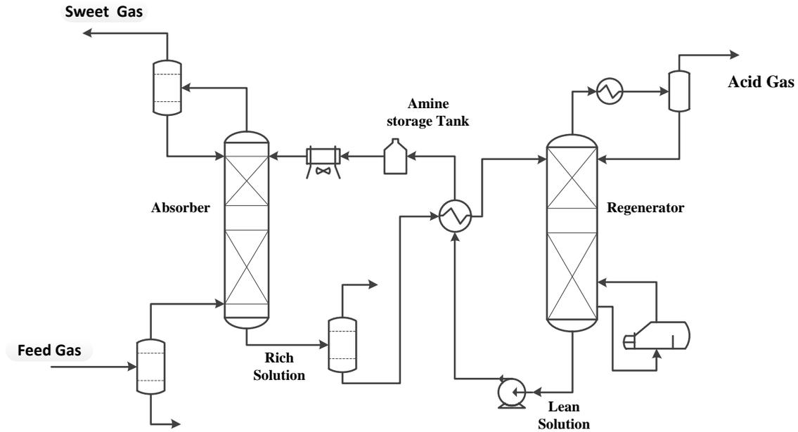
**Figure 2:** Schematic Process Flow Diagram for an Amine gas treating plant
