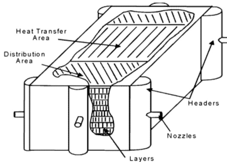
Figure 1. Brazed Exchanger Core.
