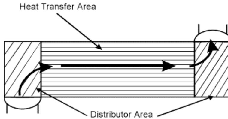
Figure 3. Heat Transfer and Distribution Areas in Brazed Exchangers.
