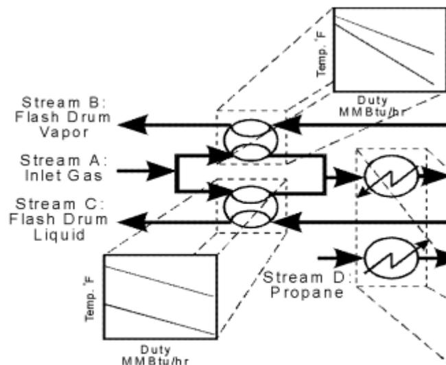
This example is a case study described by Polasek *et al.*<sup>12</sup> Inlet gas is cooled and condensed by the vapor and liquid portions leaving a flash tank. Additional cooling is provided by propane refrigeration. The original case was modified to better represent an actual design. The inlet gas flow rate is increased by an order of magnitude and the propane refrigeration is heated to 1 degree of superheat rather than to 110°F.
