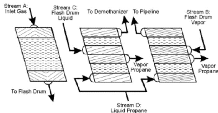
Figure 10. Stacking Arrangement and Fluid Routing for Case 4.
