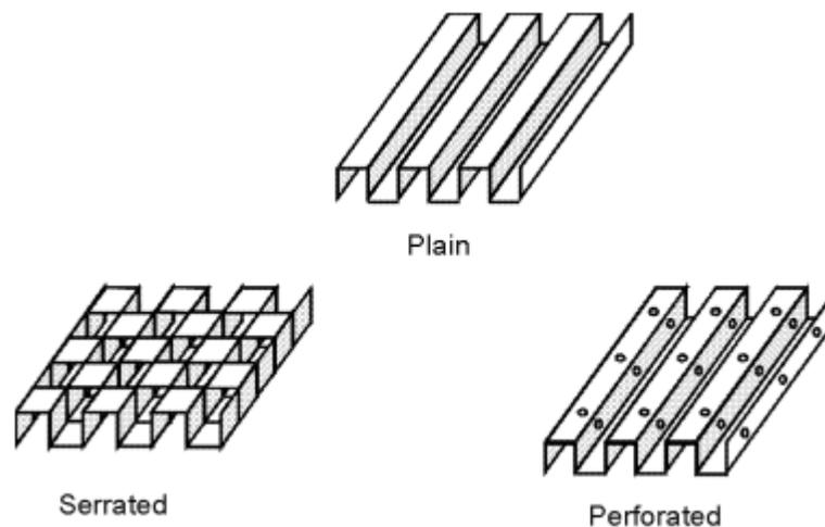
Figure 2. Types of Fins for Brazed Exchangers.
