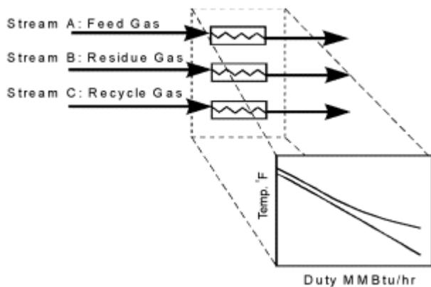
Figure 8. Duty versus Temperature for Case 3 with Shell-and-tube Network.
